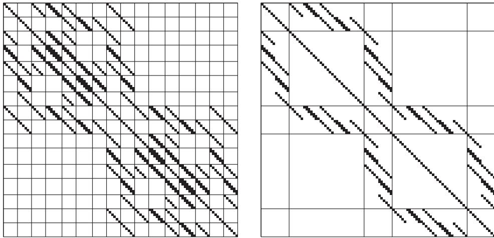
**Figure 4.** Sparsity structure of matrix  $A$  (left) and matrix  $B$  (right) for division of  $\Omega$  into  $2 \times 2 \times 6$  hexahedrons. Non-zero elements are marked as small squares
