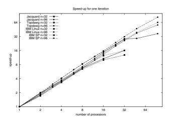
Fig. 3. Speed-up for one iteration on the parallel computer systems
