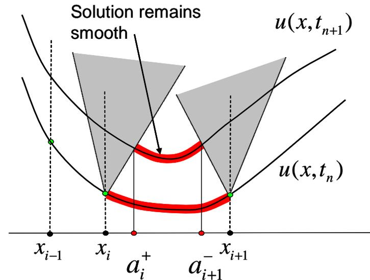
$$\begin{aligned} \frac{du_i}{dt}(t_n) = & - \frac{a_i^- H(u_x^+) + a_i^+ H(u_x^-)}{a_i^+ + a_i^-} \\ & + a_i^- a_i^+ \left[ \frac{u_x^+ - u_x^-}{a_i^+ + a_i^-} - \text{minmod} \left( \frac{u_x^+ - \tilde{u}_x}{a_i^+ + a_i^-}, \frac{\tilde{u}_x - u_x^-}{a_i^+ + a_i^-} \right) \right] \end{aligned} \quad (3)$$
