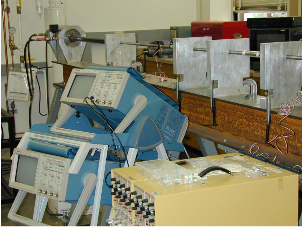
Fig. 12. Photograph of the Hopkinson bar experimental setup. The specimen is visible at the top-right part of the photograph
