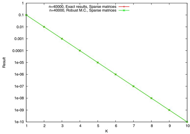
**Fig. 5.** Comparison of the MC results for bilinear form of matrix powers for a sparse matrix of size  $n = 40000$  with the exact solution
