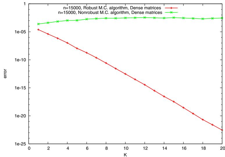
**Fig. 2.** Comparison of the Relative MC error for the robust and non-robust algorithms. Matrices of size  $n = 15000$  are used.
