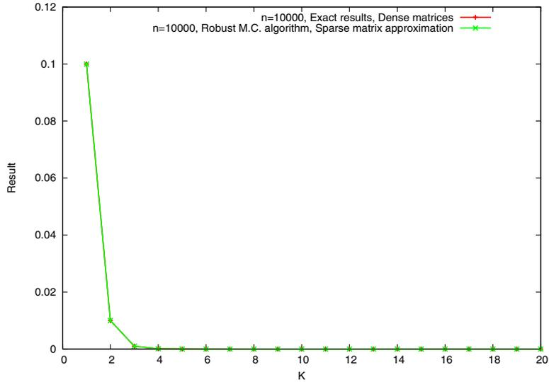
**Fig. 4.** Comparison of the MC results for bilinear form of matrix powers for a sparse matrix of size  $n = 10000$  with the exact solution. 5 or 6 Monte Carlo iterations are enough for solving the system of linear algebraic equations or for computing the dominant eigenvalue for the robust Monte Carlo.
